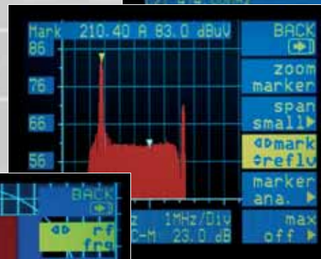
RF spectrum of an analog TV signal
